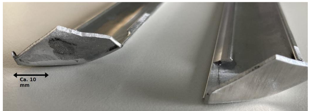
Profile with drawn edges before final machining
