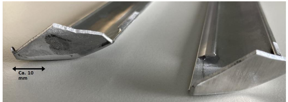
Profile with drawn edges before final machining
