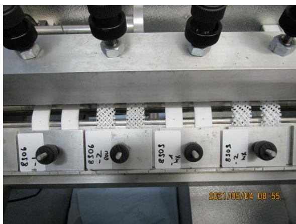
Test set-up of Ross flex measurement of Ultrasint® TPU 90A LT
