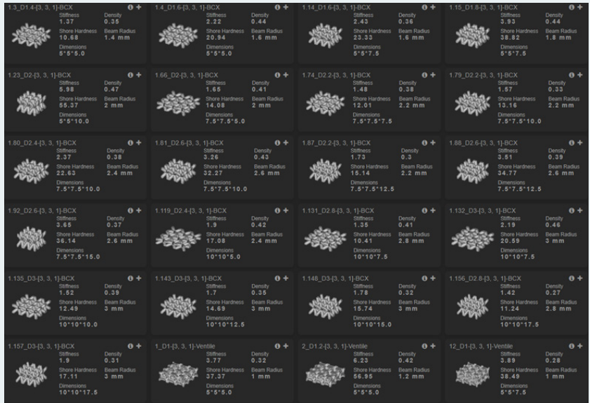
Image 7: Digital lattice library generated with Ultrasim®'s Automated Workflow (Source: Forward AM).
