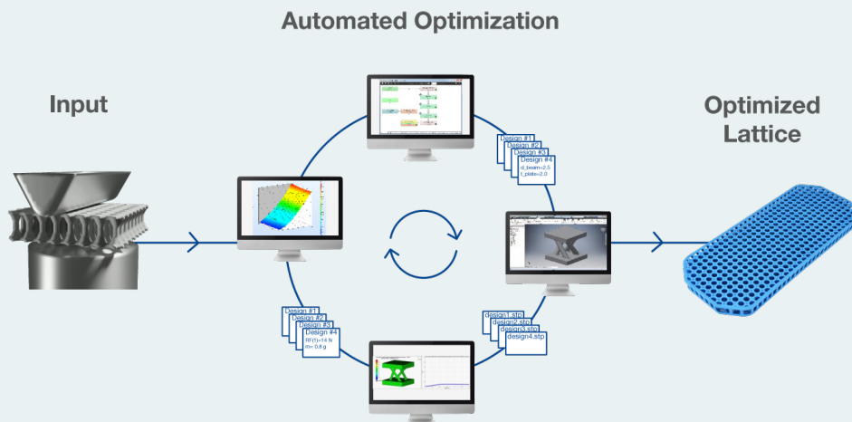
Image 6: How to virtually engineer the ideal lattice: After identifying an application's requirements and functional demands, the ideal match is generated in Ultrasim® (Source: Forward AM).
