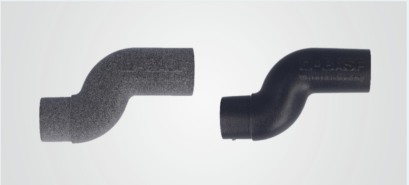
Figure 1: Piping duct printed with Ultrasint® TPU01 before and after chemical vapour smoothing.
