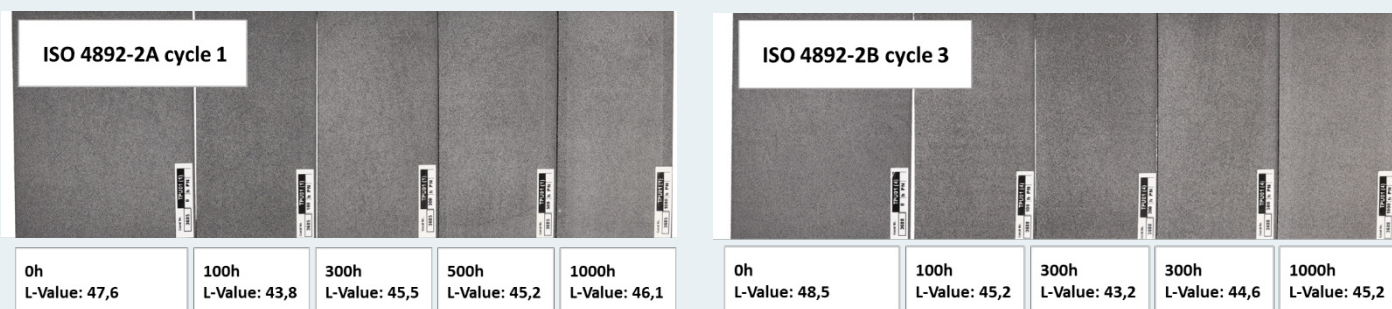
Image 4: Colour fastness of sandblasted Ultrasint® TPU01 samples from 0h to 1000h (Source: Forward AM).
