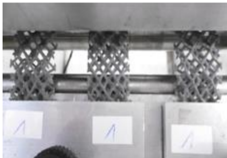
Test set-up of Ross flex measurement of Ultrasint® TPU01
