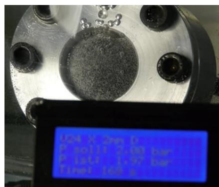
Test set-up for measuring air tightness
