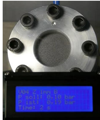
Test set-up for measuring burst pressure
