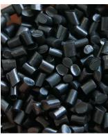
■ Virtucycle® program is about reengineering and recompounding high performance long-chain polyamides at the Arkema Agiplast plant in Italy for example in pellets for injection molding applications like automotive, sports, consumer market, etc
