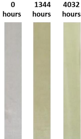
*Figure 3 Effect of UV exposure on color of the specimens*
