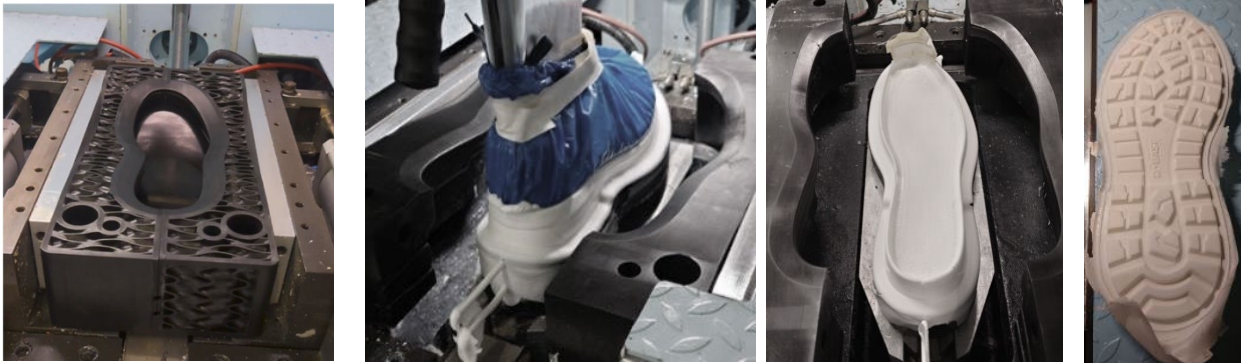
3D-printed insert in base mold. From left to right: assembled 3-piece mold, open mold after injection, midsole after last removal, outsole profile after removal
