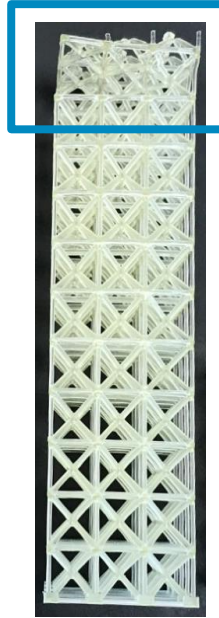
Fig. 6. Fail long lattice EL 60 - BCC - 1mm
