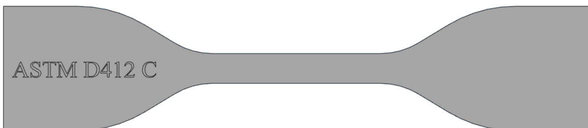
Figure 1 Tensile bar ASTM D412 Type C
