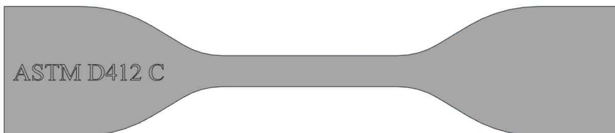
Figure 1 Tensile bar ASTM D412 Type C
