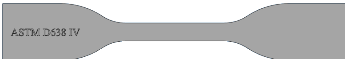
Figure 1 Tensile bar ASTM D638 IV
