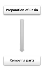
The material should be processed at room temperature. Before usage the material should be shaken well. Pour it slowly in the vat and wait a couple minutes, until smooth, bubble-free surface is obtained before starting the print job.
