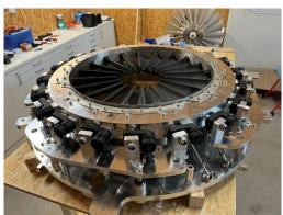
VentoStream used Forward AM's Ultrafuse® PAHT CF15 to 3D print parts that are both strong and lightweight. This high-performance polyimide contains 15% carbon fiber and resists UV light, aging, outdoor temperatures, and weather. It's also ESD safe and supports the prototyping and production of complex parts with geometries, such as lattices, that traditional manufacturing can't achieve.
