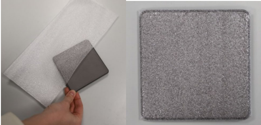
Figure 3: Wrapping the shrinkage plate in the film
