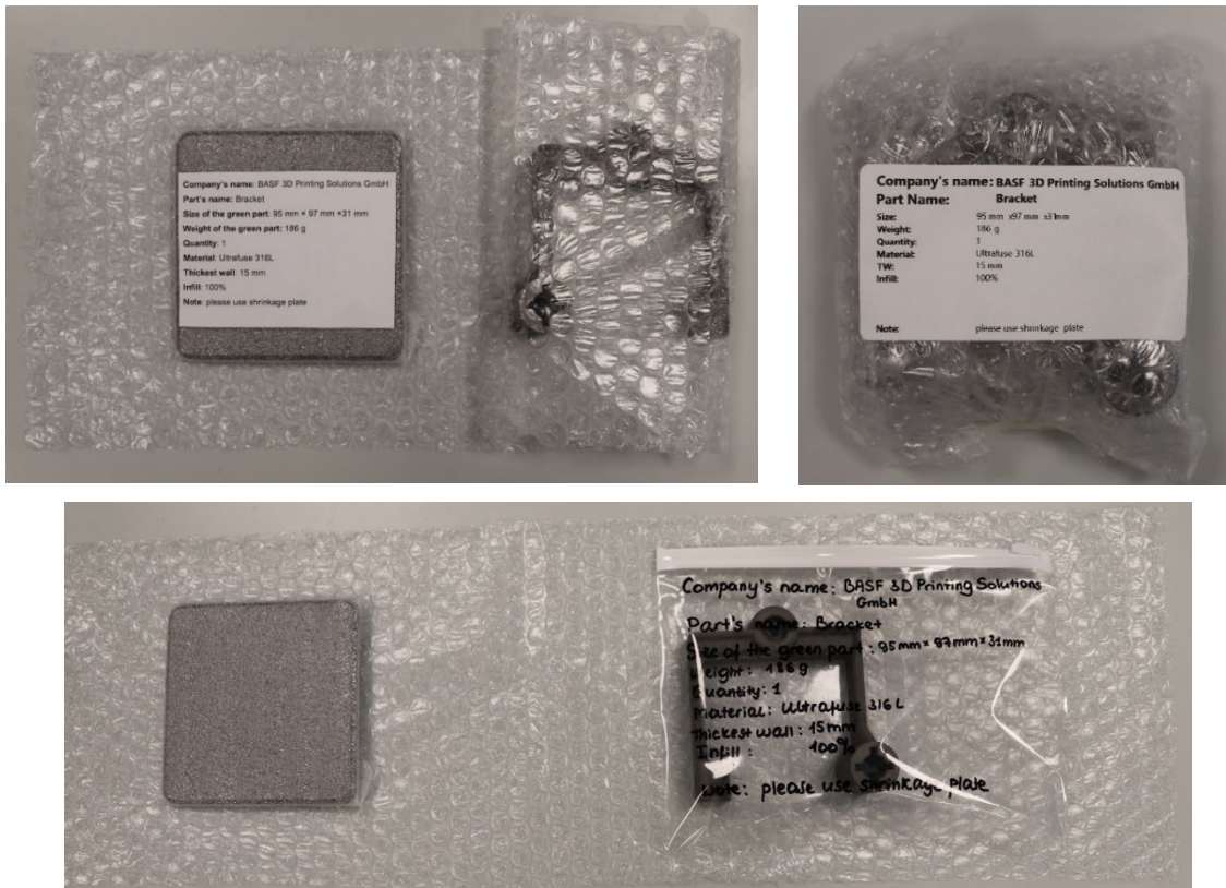
Figure 7: Different possibilities of parts labelling: adding a note (top left); using a printed label (top right); labelling with a foil pen (bottom).
