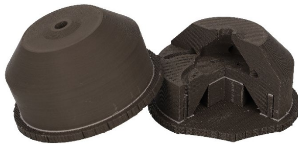
Figure 1: Greenpart with support layer and raft (shrinkage plate)
