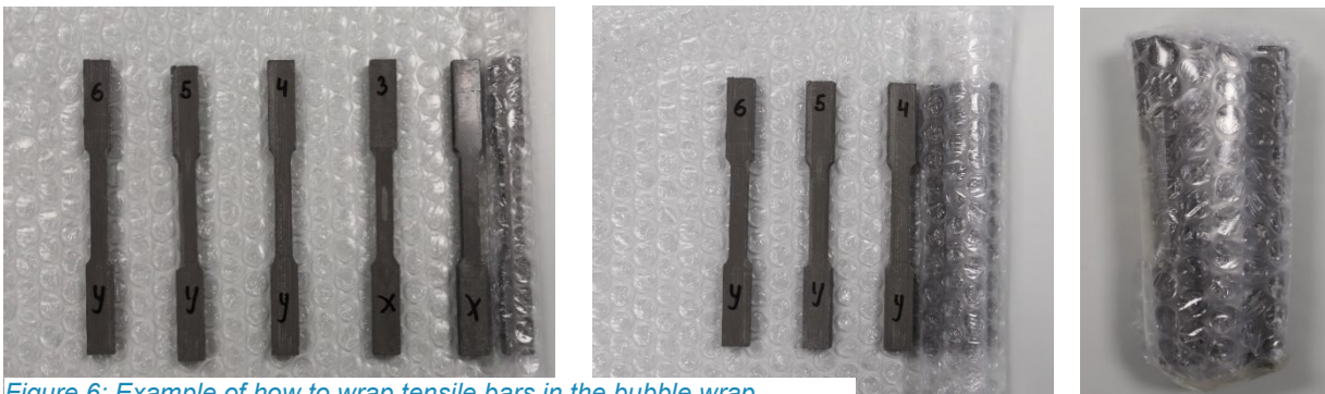
Figure 6: Example of how to wrap tensile bars in the bubble wrap
