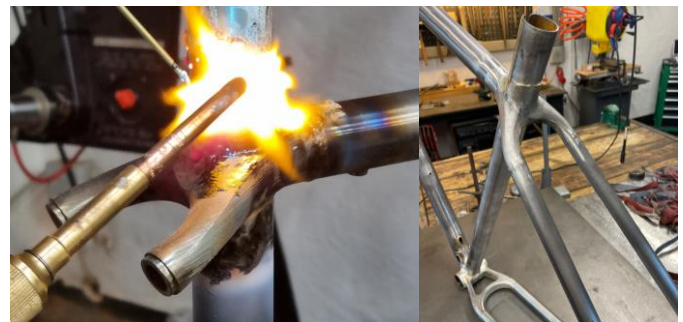
Welding Ultrafuse® 17-4 PH Connector
